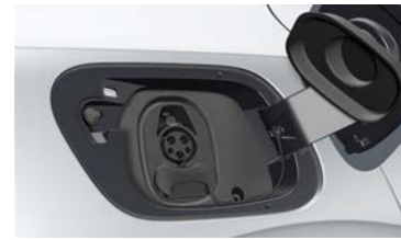
Charging socket Type 1 AC (e.g. in NAR, South Korea, Japan)
