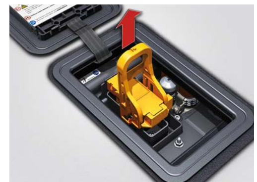
Fold the lever upwards and pull the connector up and out.
