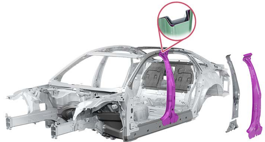
B-pillar with multi-shell structure
