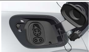
Charging socket CCS1 DC and AC (e.g. in NAR, South Korea)
