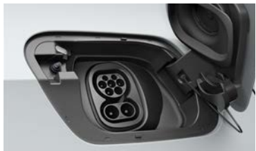
Charging socket CCS2 DC and AC (e.g. in the EU)
