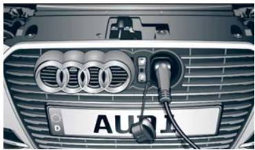
A3 “e-tron” charging socket (2014 to 2020) on the radiator grille
