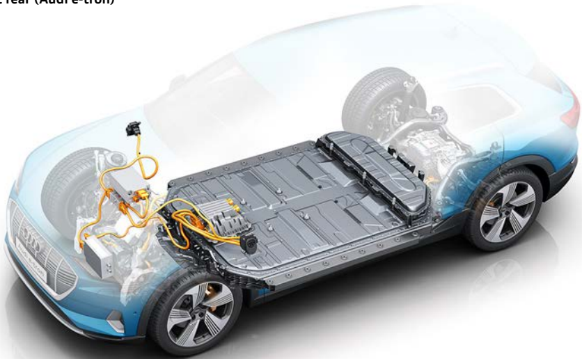
High-voltage battery in vehicle floor with additional package at rear (Audi e-tron)
