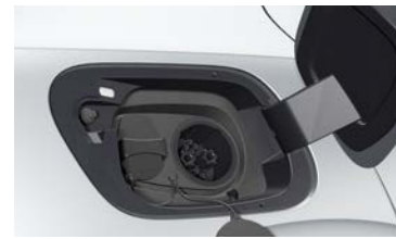
Charging socket CHAdeMO DC (e.g. in Japan)
